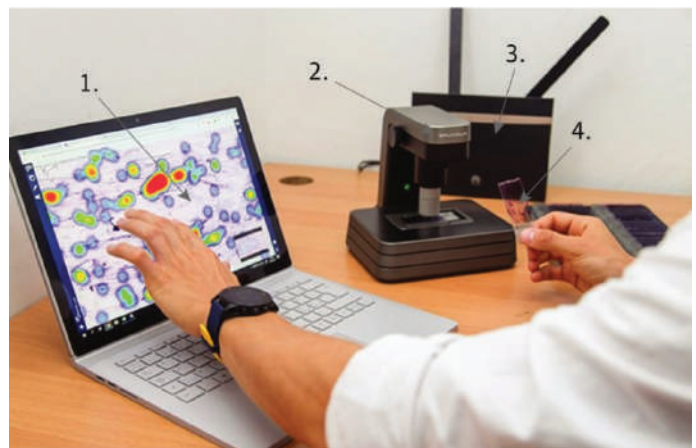
Figure 6: Slide digitization equipment, including (1) laptop computer with access to the slide-management platform, (2) slide scanner, (3) mobile-network router, and (4) Papanicolaou test microscopy slide Image source: Holmstöm et al., JAMA Network Open 2021.
